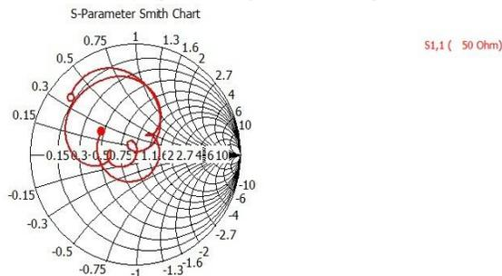
Figure 3:-Smith chart plot (microstrip line feed) for simulated antenna design
