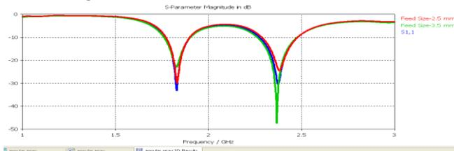
Figure 7 – Effect of feed width ( $\epsilon_r$ ) on antenna performance characteristics
