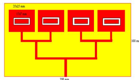
Fig. 1 The proposed Microstrip antenna array
