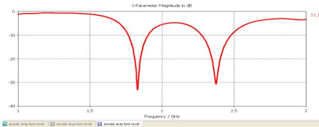
Fig.2.The reflection coefficient (S11, dB) versus frequency (GHz) plot for antenna design.
