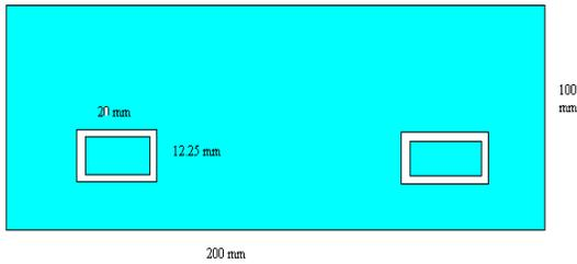
(b) Ground Structure of Antenna Array
