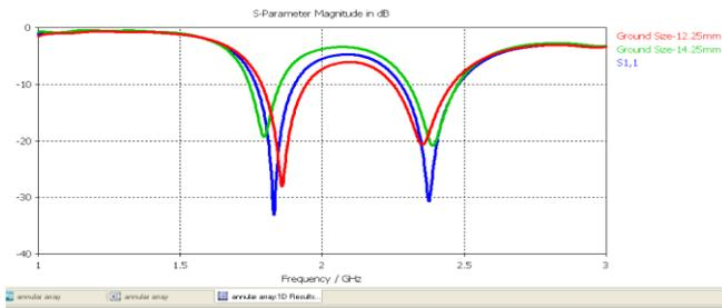
Figure 6: Effect of ground size variation on the antenna performance
