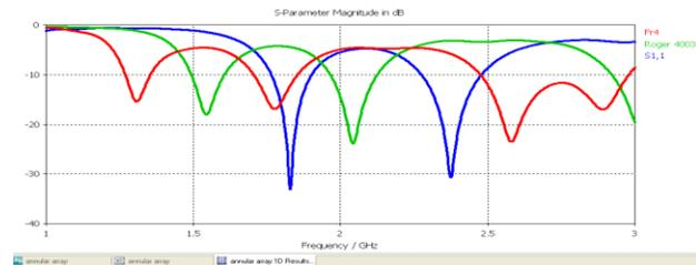
Figure 4: Effect of substrate material on the antenna performance
